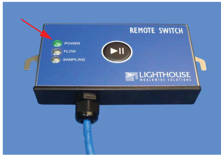
Figure 3-15 Remote Switch with Power
