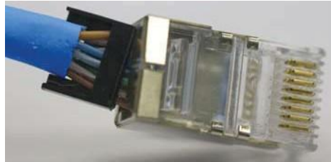
Figure 3-5 Loomed wires inserted into RJ-45
