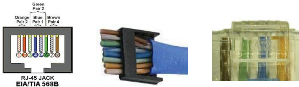
Figure 3-4 EIA/TIA-568B Color Code Example
