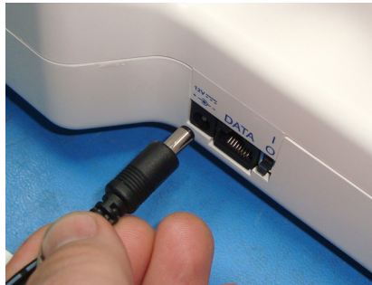
Figure 3-7 DC Power Plug
