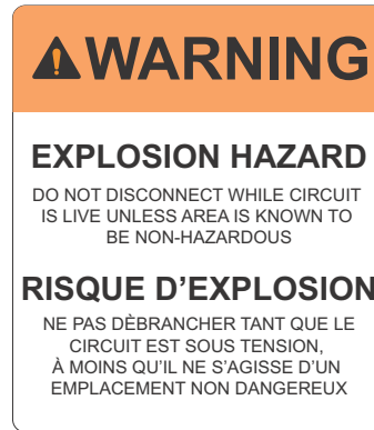
Figure B-1 Explosion Hazard Label
