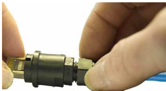
Figure 3-10 Tighten Cable Clamp Nut
