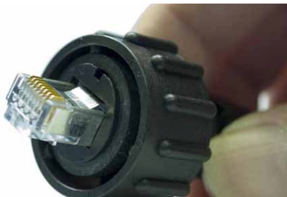
Figure 3-12 Cable Connector Completed
