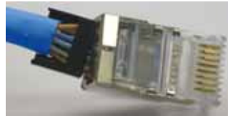
Figure 3-5 Loomed Wires Being Inserted into RJ-45
