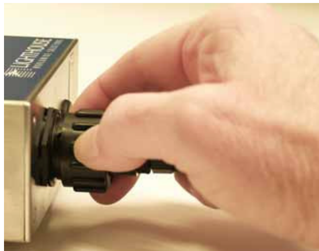
Figure 3-20 Cable Fully Attached
